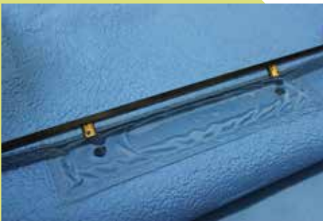
Indexing holes for fixing with indexing bars
